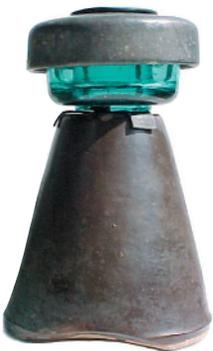
The oil insulator / earthenware pedestal was used to support a battery tank that was constructed of wood and lined with lead. The exterior was coated with asphaltum. Four to six CD-35s or CD-36s were used to support this style of Battery Tank.
