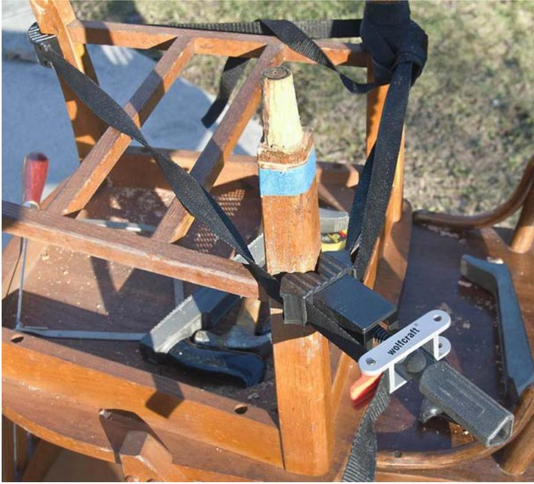
This is a strap clamp. It is made for holding all four corners of a four-cornered object in place during gluing. For the present purposes, its function is to hold in a relatively stable position the one leg which is being chiseled, and to prevent the hammering shocks from breaking down the glue joints of the chair.
