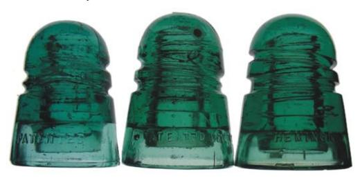
Typical BROOKFIELD, HEMINGRAY Type #5, typical HEMI Note the BROOKFIELD like rounded features, height and the color of the middle HEMI #5s while retaining the HEMINGRAY style taper.
